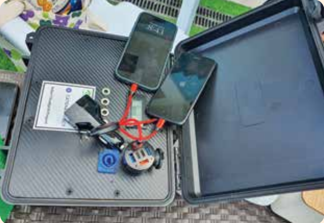
Solar-powered battery unit charging phones.
